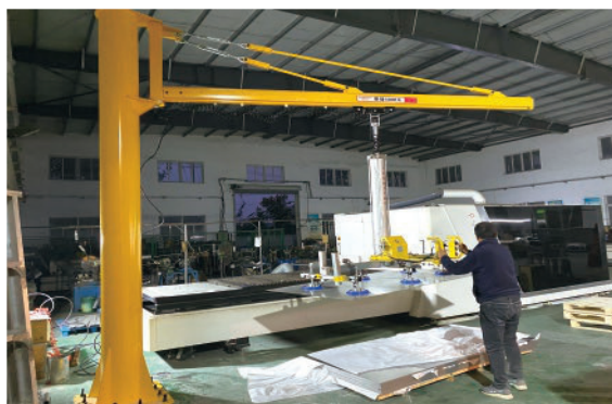
Manual Swing Arm - Manual Walking AL-LZ-500KG
