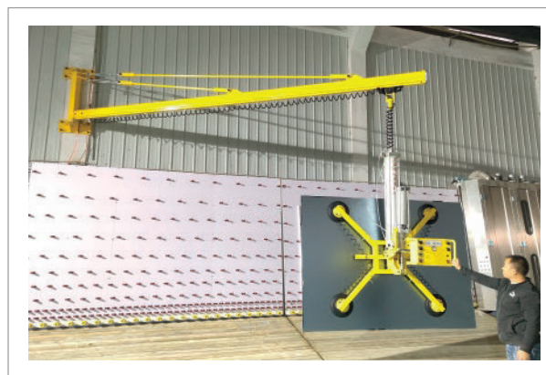
Manual Swing Arm-Manual Walking AL-QB-500KG
